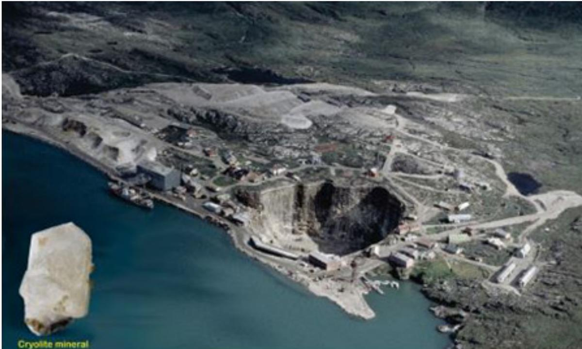
Ivittuut and the cryolite mine in 1960, showing working open-pit, mine infrastructure, ore and waste dumps and ship-loading facilities.
