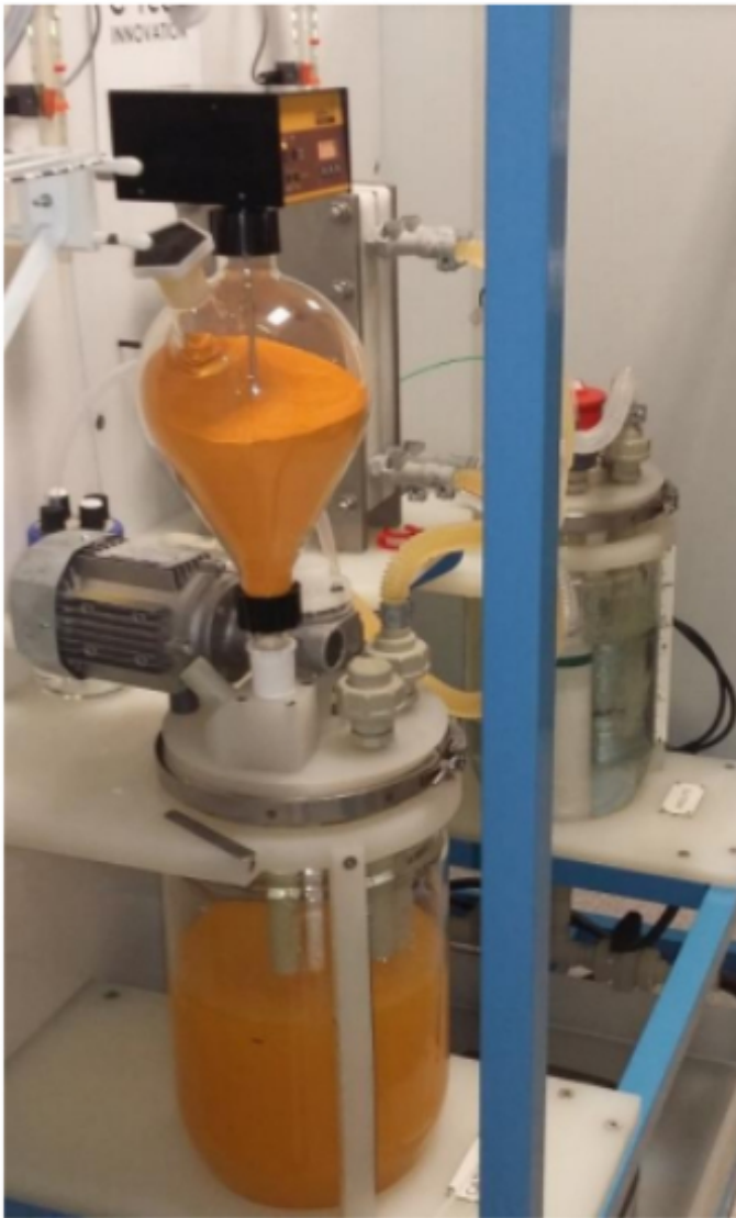
AVL's vanadium electrolyte pilot plant
