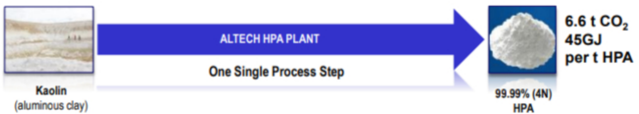
Figure 2 – Altech’s Kaolin-Alumina Process
