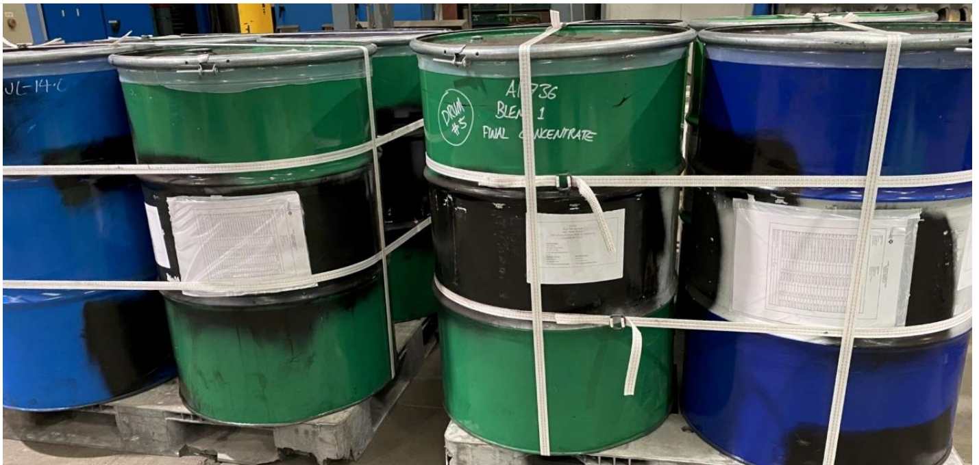
Two-tonne sample of beneficiation circuit concentrate shipped to the US for Grate Kiln pilot testing
