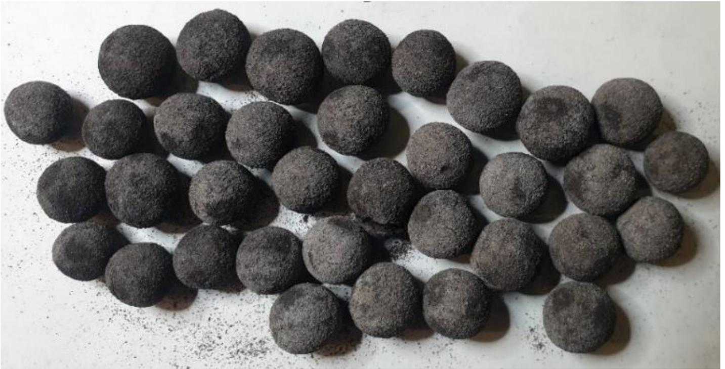
Vanadium rich iron concentrate pellets produced during bench-scale roast testing
