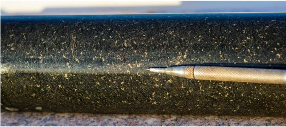
Drill core with heavily disseminated sulphides from 46.3 metres to 48.7 metres downhole in MAD152 at the Radar Prospect
