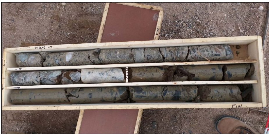
C201219, at ~273 metres showing brine bearing breccia/conglomerate host lithology
