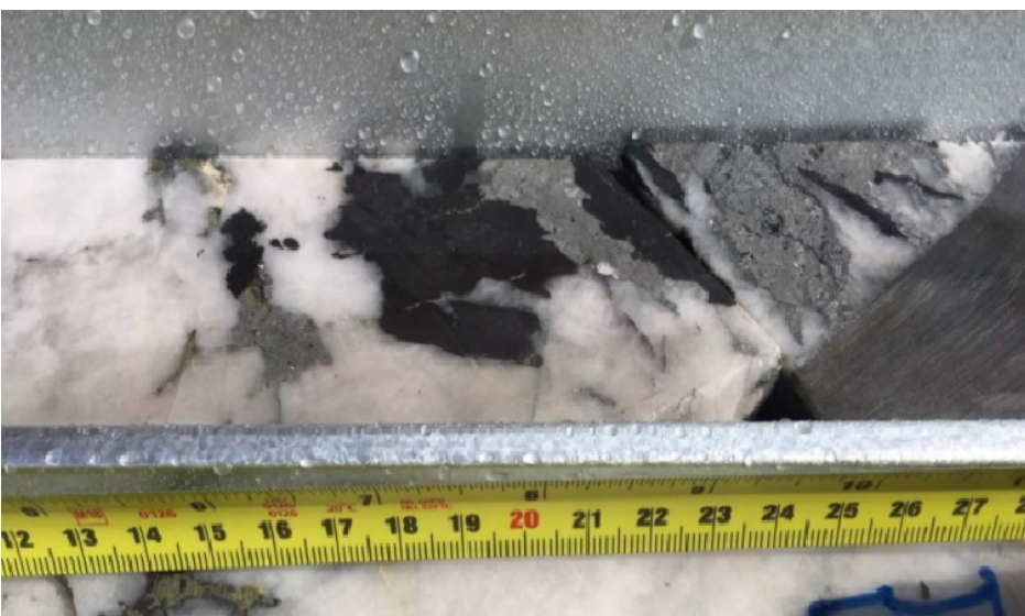
Wolframite in quartz vein, from 432.4 metres
